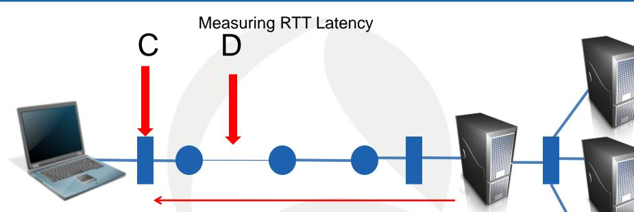
C - Taking capture trace before the router D – At the same time capturing after the router
